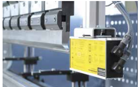
CE Laser Safety System
