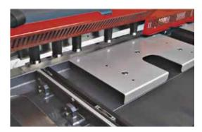
Flip-up Finger Guard Adjustable Ball Transfer Table Hydraulic Holddowns
