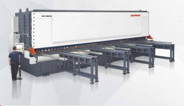
Sheet Support + Belt Conveyor + Stacker + Scrap Container
